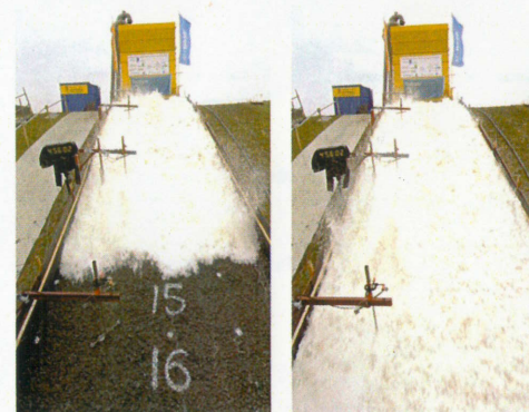
Elastocoast® revetment tested against overtopping by Rijkswaterstaat (NL) showed outstanding performance
