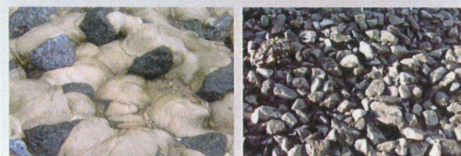
Concrete revetment Open stone asphalt
